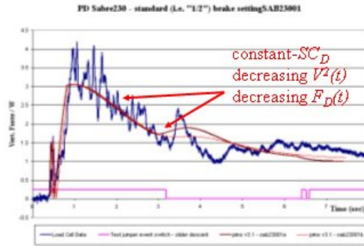
Figure 4. Riser load evolution graph for a skydiving parafoil, namely a Performance Designs Sabre 230 carrying a 200lbs payload. This example highlights the rare constant- SC_D slider-up inflation mode.
